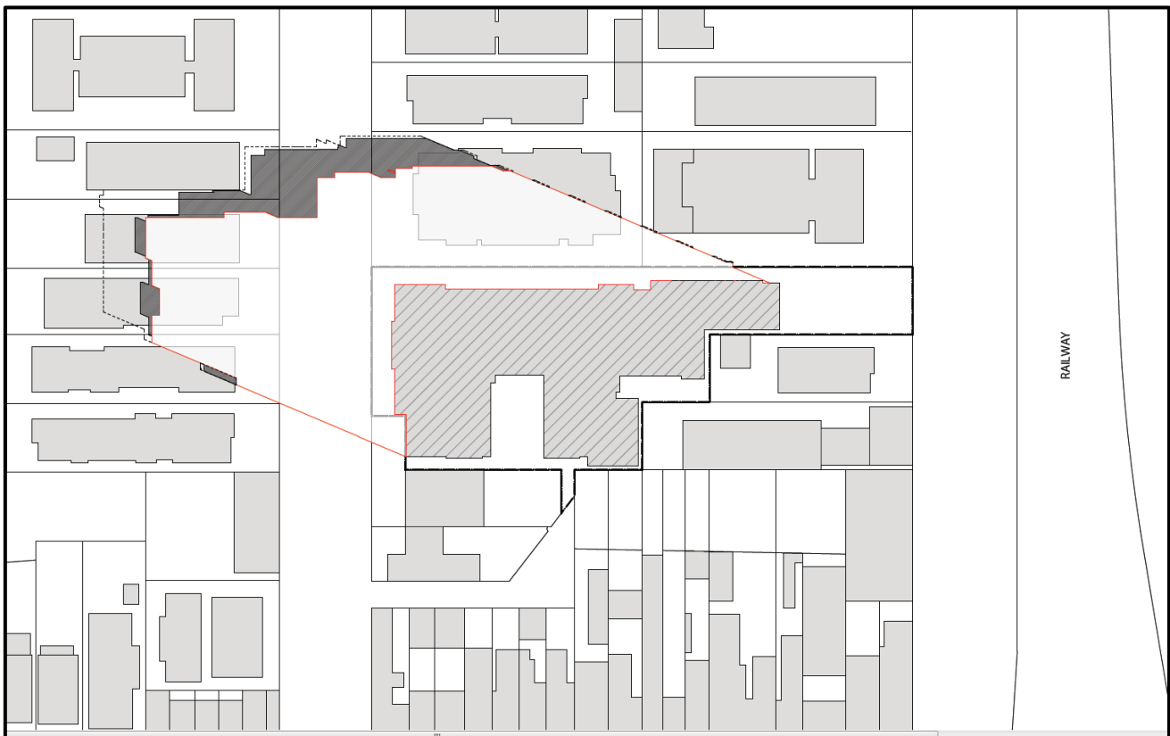
Figure 3: Shadow cast by the proposed development at 9am at the Winter Solstice.
