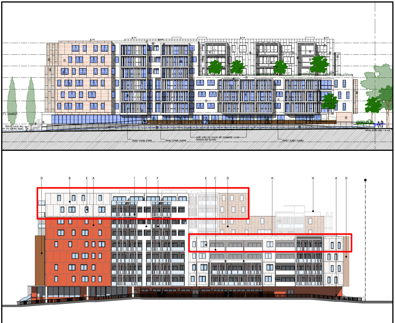
Figure 2: Approved and proposed western elevation of the development shown top and bottom respectively. The red box annotates the additional building height proposed under the subject application.
